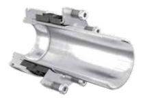
This single mechanical seal is tailored to the seal installation space of the pump. Its large external springs are insensitive to contamination and provide uniform surface pressure across the contact faces, thus ensuring a long service life. Optionally, this seal is available as a 4KD double seal.
